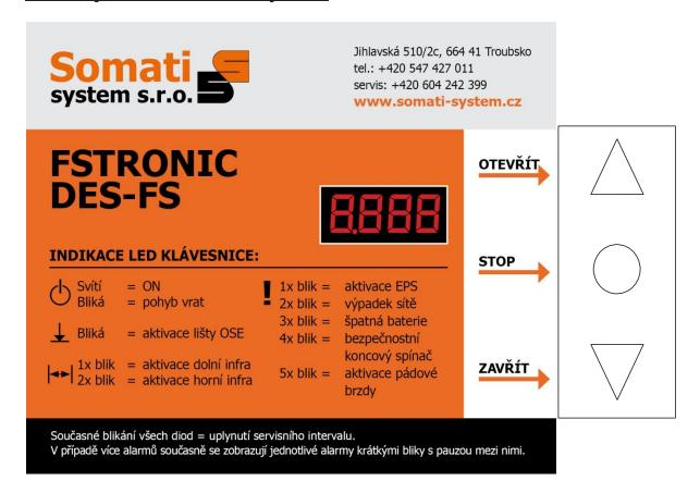
On control panel of FSTronic there is installed keyboard with buttons OPEN, STOP, CLOSE. On the keyboard there are also LED diodes, which display all current states of the control. This enables the gate operator to determine particular states and potential gate alarms.
