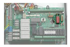
**DIP3** – activates automatic closing after opening by pressing "open" button on the keyboard of control panel, "open" button has same function in case of activation as pull switch (i.e. after setting time in parameter "6", gate is automatically closed)
