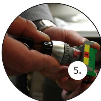
**!** Do not connect any external controls or any other devices before setting the end switches – it can cause automatic start, which is not restricted due to the unset end switches.
