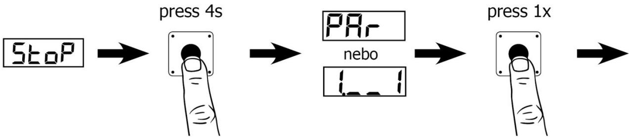
Description of setting of optional parameters on display device. To enter the setup we have to hold knob button and after 4 seconds display shows „Par” „Par” /or 1 \_ \_ 1 (0) – direct display of parameter No.1 – valid for versions supplied until 04/2015.
