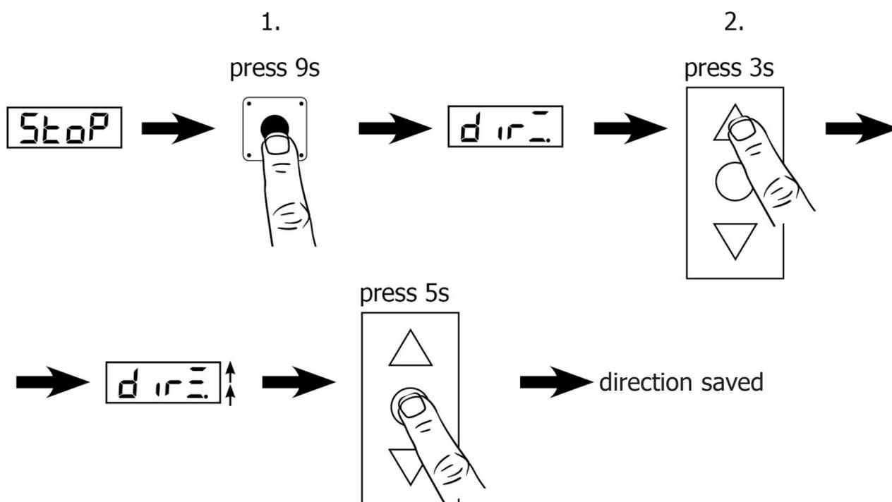
Setting is possible only from STOP state, "stop" must be shown on display.
