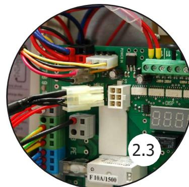
3. **Connect terminals EPS** (X2:+ and X:10) NC contact (in case the contact is disconnected, gate is constantly closing in alarm). Originally delivered with connection "fire contact".
